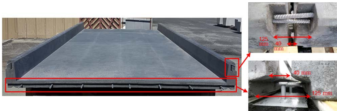
Figure 1. UHPFRC precast slab and field-cast joint geometry
