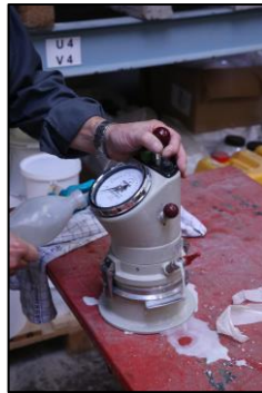
Figure 3. Equipment for measuring fresh density and air content
