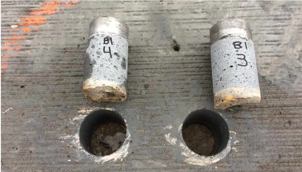
Figure 1. UHPC-Concrete Bond Test Samples After Testing
